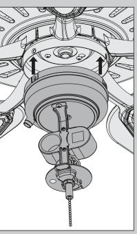
Lift the lower switch housing up until the screw holes line up with the screw holes in the upper switch housing.
